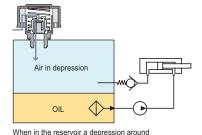
0.030 bar is produced, a flux of air entering the reservoir through the suction valve takes place.
